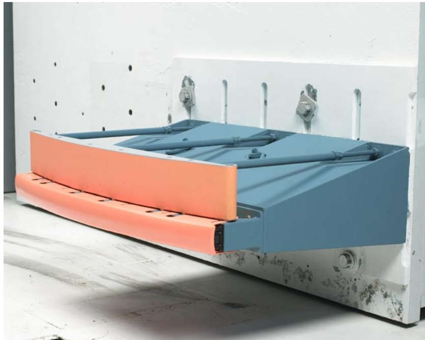
Figure 6 Plastic Energy Absorber and Cover Mounted on Bumper Barrier
