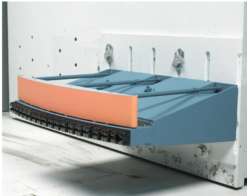
Figure 4 Plastic Energy Absorber Mounted on Bumper Barrier
