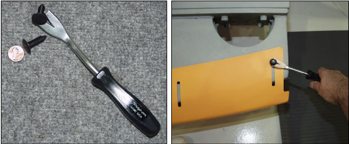
Figure 5 Nylon Push-Pin Rivet Fasteners (McMaster-Carr Part #90221A119)
